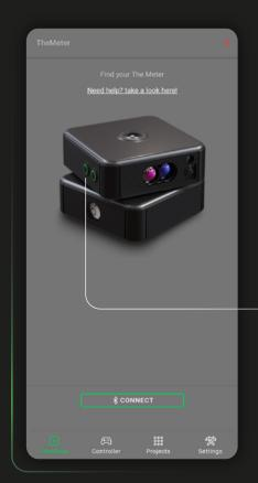
With this mode you can perform surveys by directly choosing which points on the surfaces to be reached and beaten; By rotating the **CUBE** PRO via The Meter App controller you can create polyline plans of your spaces, avoiding clutter and elements you don't want to have in the resulting DXF file
