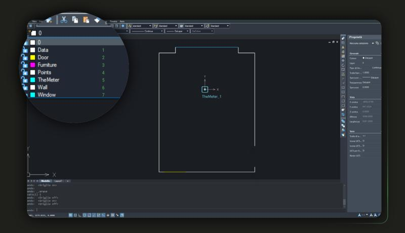
The drawing is divided into several levels: in "Data" you will find the generic data associated with the file, in Door<sup>2</sup>, Furniture<sup>3</sup>, Points<sup>4</sup>, Wall<sup>6</sup> and Window<sup>7</sup> the polylines with which you have created the scan, in "TheMeter" <sup>5</sup> the location of **CUBE**<sub>PRO</sub>
