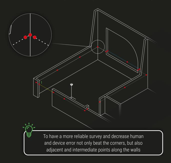
During the construction of the survey, the app shows you on screen the project development following the point of view of **CUBE**<sub>PRO</sub>
